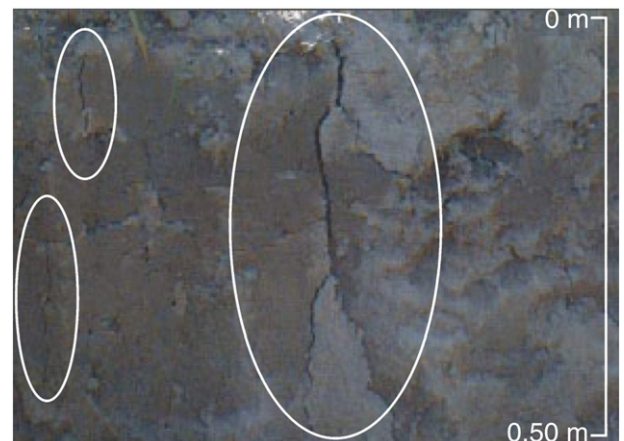
Fig. 9. Illustration of cracks in moderately dry soil (MD) following the passage of the machine from left to right.
