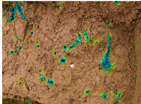
Fig. 3. Transversal section at 0.30 m depth showing the limited interaction between macropores and matrix in the silty clay material.
