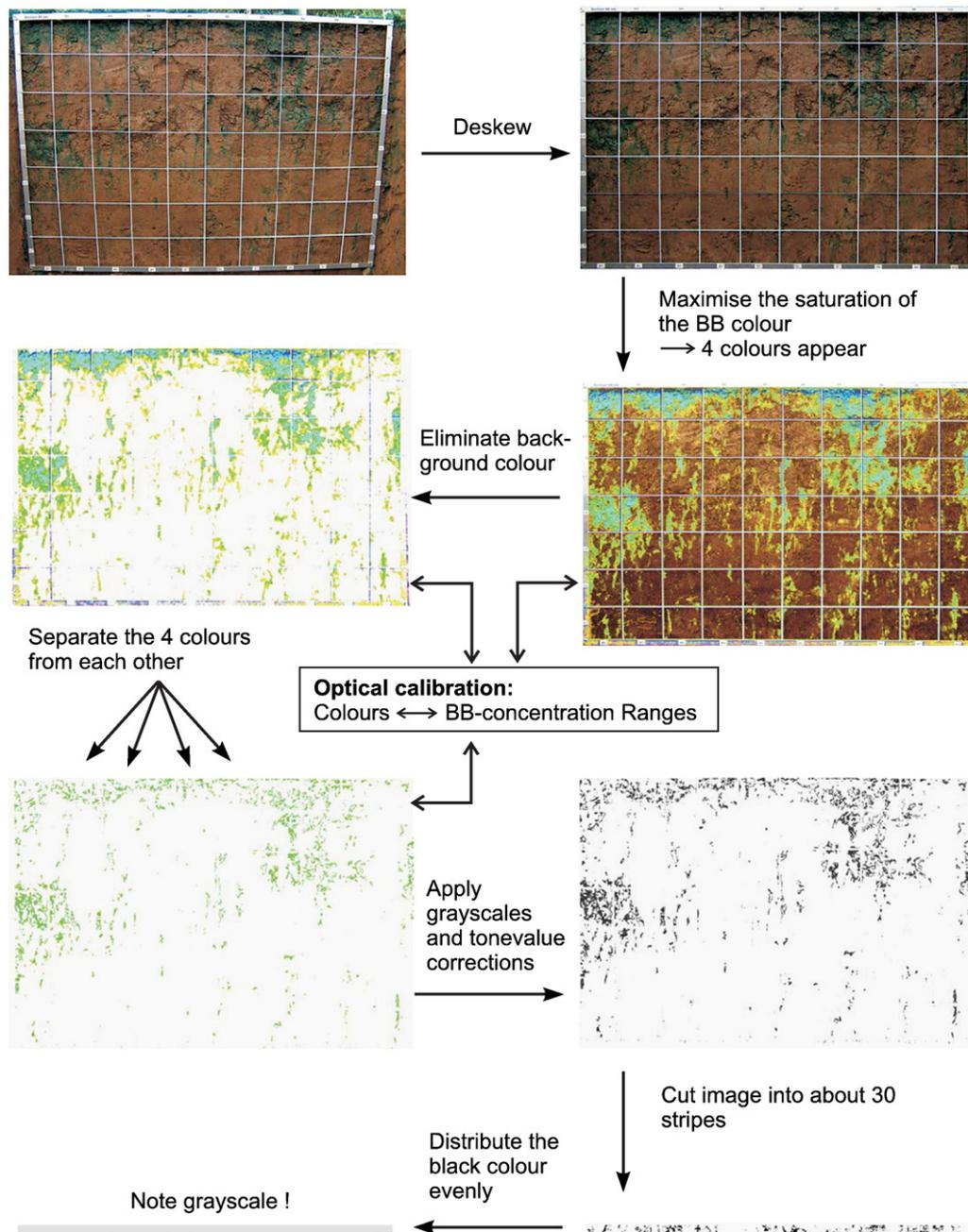
Fig. 1. Schematic illustration of the image analysis procedure in order to obtain diagrams out of images using Photoshop CS2®.
